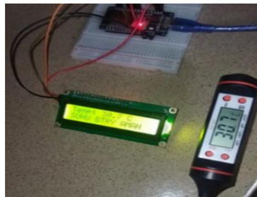
Gambar 5. Kalibrasi sensor suhu
